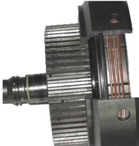
Using air (40 PSI) apply the rear clutch several times to seat all of the clutch pack elements. With a feeler gauge, measure between the bottom of the selective snap ring and the top of the pressure plate. Clearance should be .025" to .050" (0.64 to 1.27mm). Clearance should be correct with the .060" (1.52mm) snap ring provided. However, there are selective snap rings available if needed.
