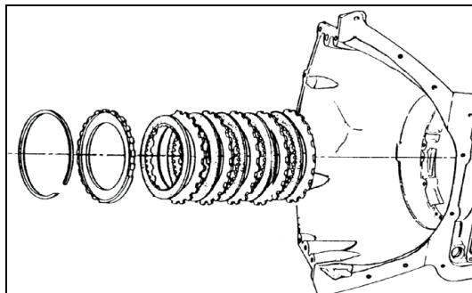
Apply air (40 PSI max) to center support port for the intermediate several times to seat the clutch pack elements. Clutch pack clearance is .040" to .107" (1.02 to 2.72mm) check with feeler gauge between the bottom of the snap ring and the top of the pressure plate.
